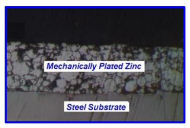
This photomicrograph of a cross-section of a mechanical plated coating shows the porous coating which allows hydrogen to escape, eliminating the risk of hydrogen embrittlement.
